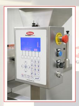
The membrane control panel allows easy access to machine and product parameters which gives the operator good visibility of the complete filling process. The product library can store up to 1000 different setups and offers instant recall of both product and machine parameters.
