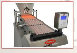
The three tray format allows the product to be progressively regulated from a bulk supply to single lines of product and contact parts are easily removed without tools and a dust extraction system allows dust to be filtered away.
